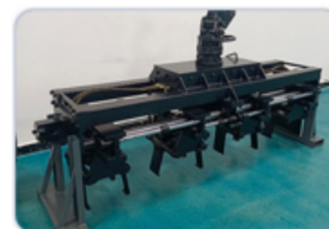
SLEEPER SPACING BEAM
